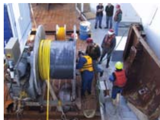
Winding on the seismic cable aboard RV Tangaroa
