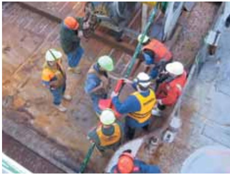
A 'bird' being attached to the streamer which is towed behind the survey ship during low fold seismic survey work. The birds help regulate the streamer's depth.
