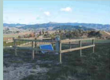
The GPS stations that make up the PositionNZ network record data every 30 seconds.
