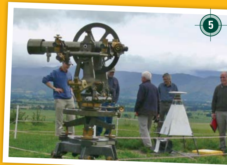
LEFT: Former Surveyor-General Tony Bevin demonstrates the use of a Model 8 Geodimeter, an electronic distance measurer, which was used extensively by Lands and Survey for survey control work in the 1970s. Looking on are (from left) Peter Chambers, Cliff Couch and Mack Thompson. (Picture: Matt Amos)
