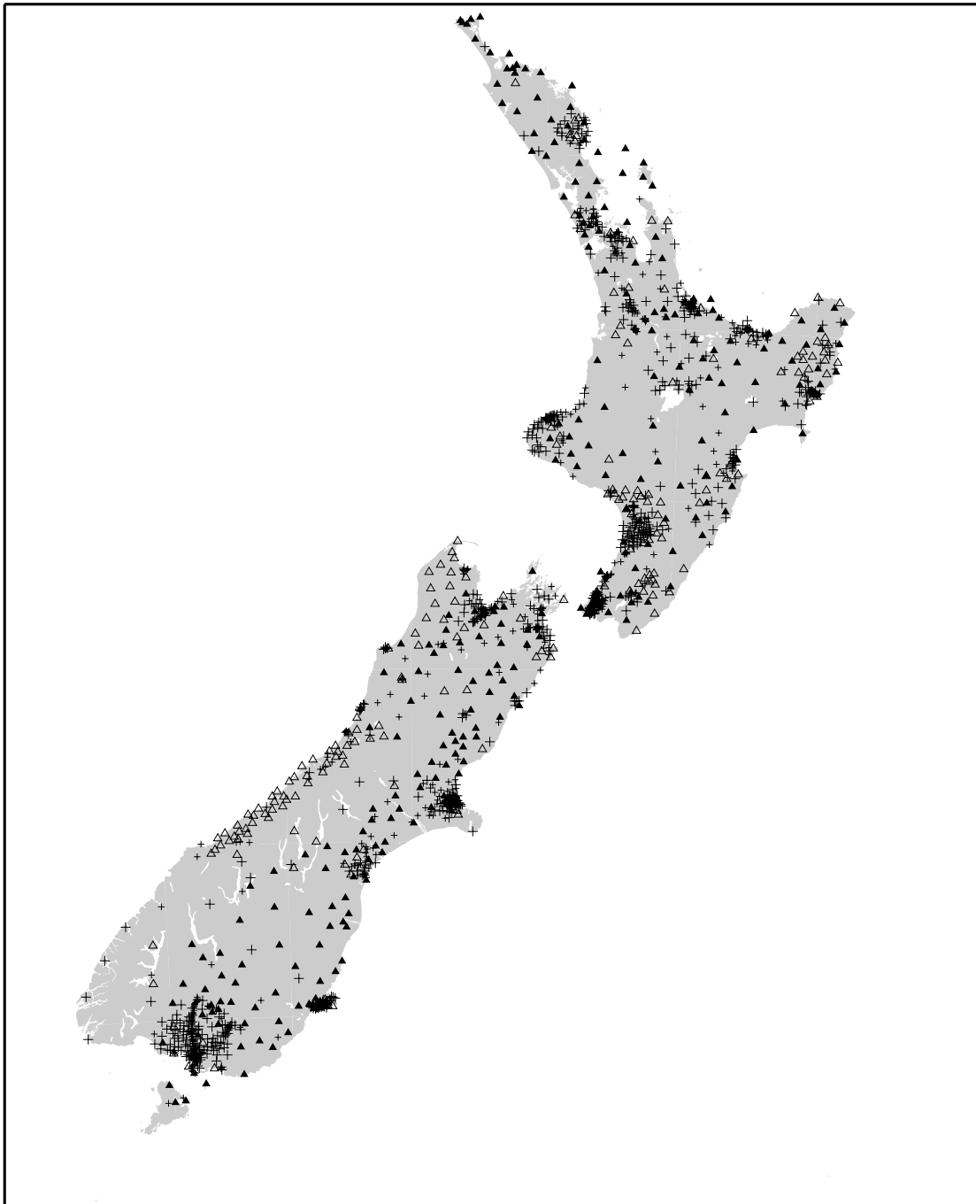
Figure 1: Control points used to calculate the NZGD49 distortion model. The symbol shows the NZGD49 order of the marks - solid triangle is 1st order, open triangle is 2nd order, large cross is 3rd order, and small cross is 4th order.
