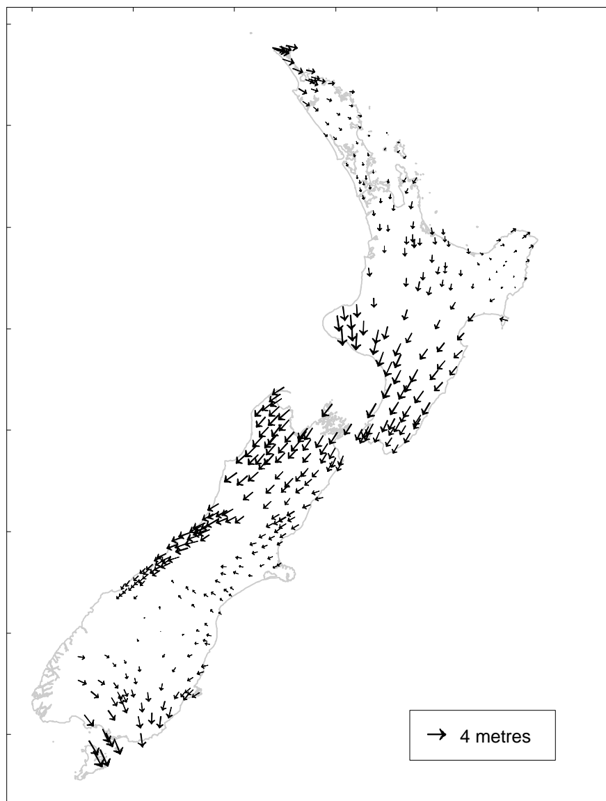
Figure 1: Shows the remaining difference between WGS84 and NZGD49 after the Mackie 7 parameter transformation has been applied to the WGS84 coordinates.
