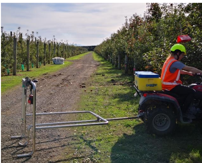
A SouthPAN enabled “rut-meter” towed by a quad bike allows Page Bloomer to accurately map rates of rut development
