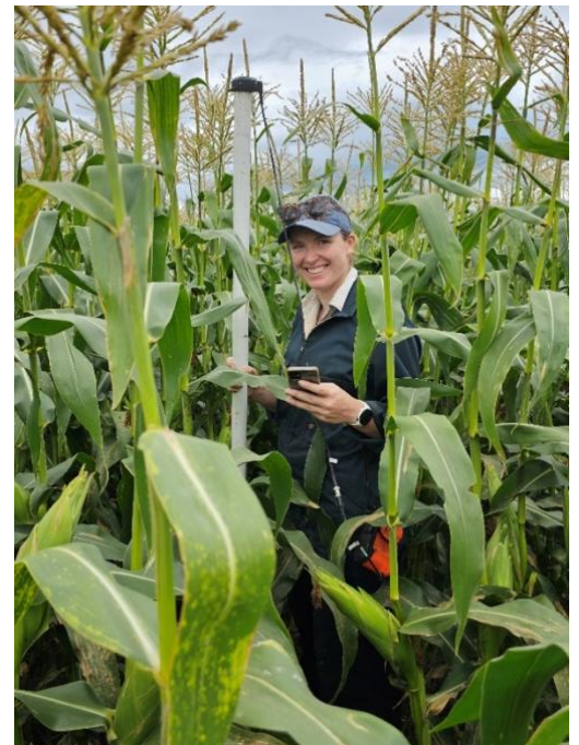
A SouthPAN enabled receiver is used to locate sampling points in maize crops, often growing up to 3 metres tall.
