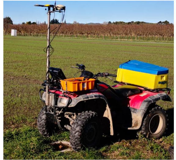
A SouthPAN enabled quad bike allows efficient and accurate mapping across a large area of otherwise inaccessible terrain.
