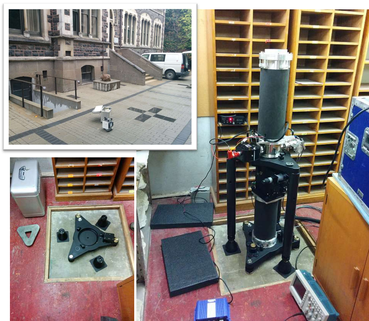
Figure 2 University of Otago Geology Department building with relative gravity meter D-37 set up on Primary Gravity Network site No. 272 (top left). The absolute gravity mark in the basement of the building (lower left) and FG5/237 set up over the mark (right).
