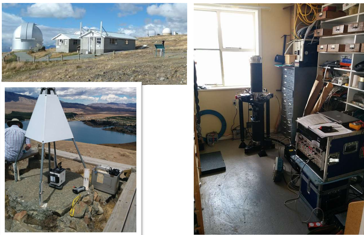
Figure 3 Mt John absolute gravity site is in the mechanical workshop (closest building in top left photo) and FG5/237 was set up in a storeroom on north side of building (right). Relative gravity meter D-37 was used to tie to mark 6702 (bottom left).
