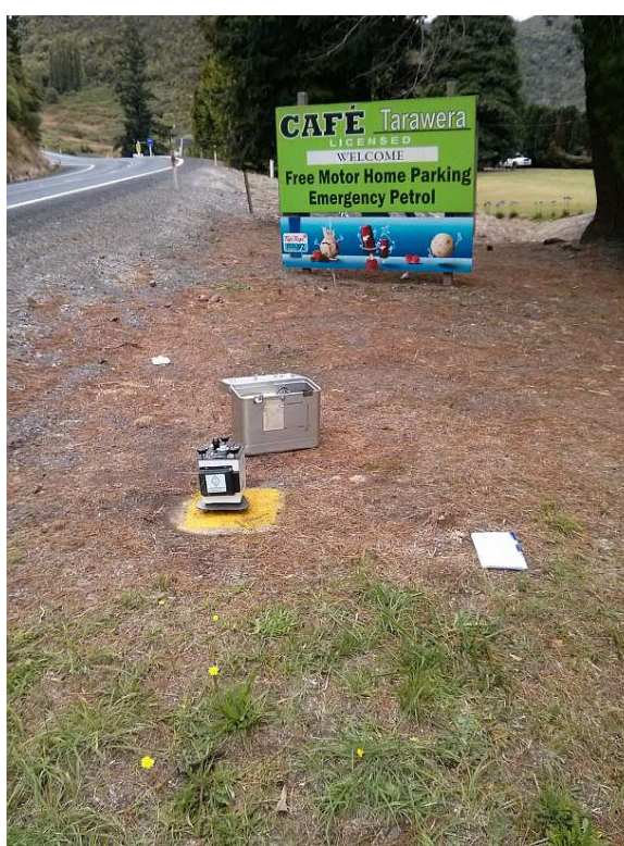
Figure 7 View of the Tarawera Café in 2015 (top), the mark is in a storage room at the back of the main building. FG5/237 set up over the Tarawera mark (lower left) and relative gravity meter D-37 on mark B401 (lower right).
