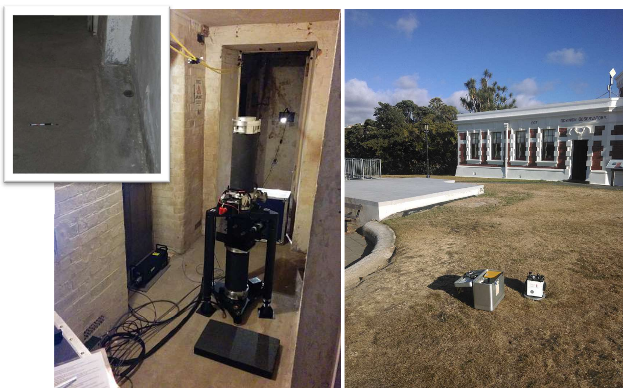
Figure 4 FG5/237 set up over the Wellington A mark (right) and inset showing the location of the mark in the concrete floor. Relative gravity meter D-37 was used to tie to mark 8105 adjacent to the Dominion Observatory building (right).
