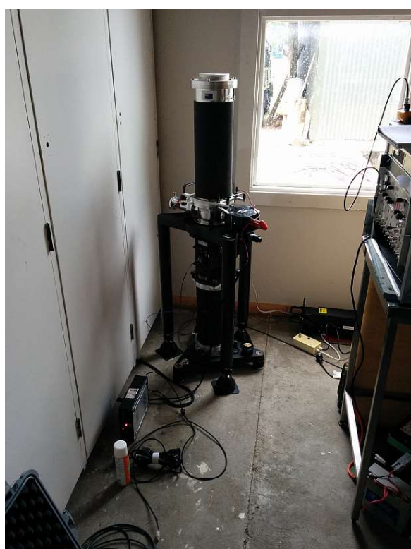
Figure 7 View of the Tarawera Café in 2015 (top), the mark is in a storage room at the back of the main building. FG5/237 set up over the Tarawera mark (lower left) and relative gravity meter D-37 on mark B401 (lower right).
