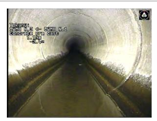
MH N.1 To MH N.2\_9edf6547-a75e-42dc-a5a2-5c82b3edac54\_20230424\_09 4747\_653.jpg, 00:00:59, 1.19m
