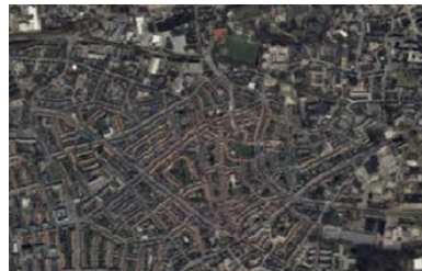
In a professionally generated orthophoto the seam lines should be almost invisible.
