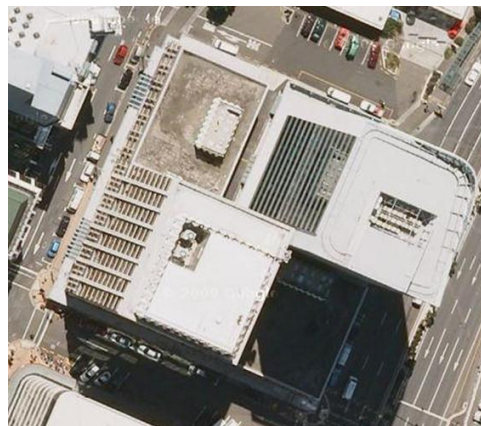
Radial displacement not removed. The top of the building obscures half of the road of the right.
