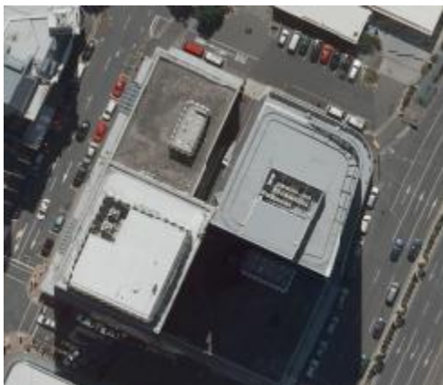
Radial displacement removed.
