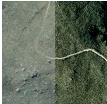
An example of where colour balancing between images has not been undertaken.
