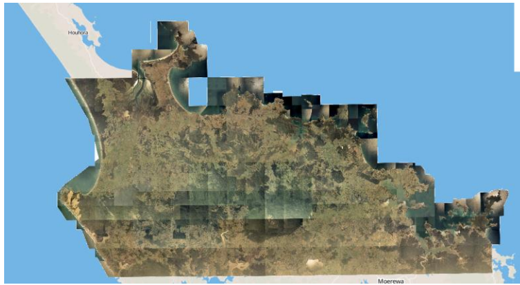
An example of where colour balancing has been applied on a per tile basis. https://data.linz.govt.nz/#layer/1907-northland-125m-rural-aerial-photos-2000/
