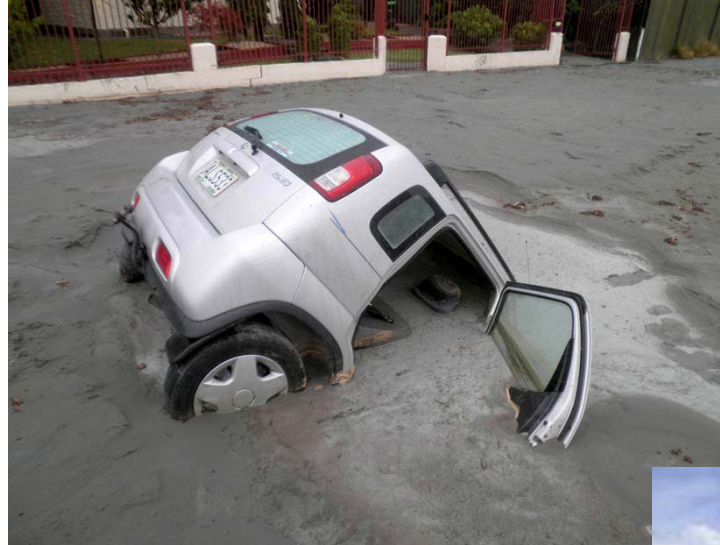
Liquefaction in Christchurch: CEISMIC Digital Archive (Mark Lincoln)
