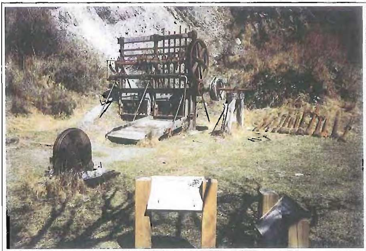
Fig. 16. Andersons stamping battery at Macetown is among the better known and more frequently visited historic remains of the goldmining era. The battery is situated within the existing small Historic Reserve which includes the township and a narrow strip up the Rich Burn. There are however, many more remote remains which could be included in a much enlarged reserve as an outcome of tenure review.
