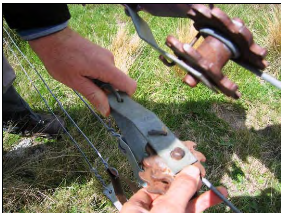
Plate 3. Hayes strainers on lower internal fence line ca.570m contour at GPS 049.
