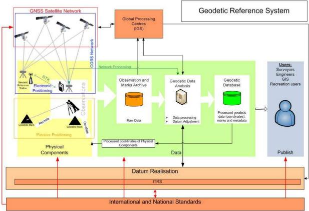
Fig 5 – Geodetic Reference System
