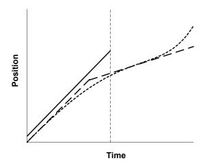
**Fig. 2.** One dimensional position of a mark against time. Dotted line shows the actual movement of the mark. The solid line is the initial deformation model and the dashed line is the revised deformation model after the time of updating, indicated by the vertical dashed line.
