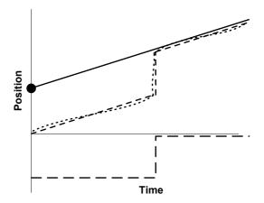
**Fig 4**. Coordinate of mark defined by deformation model incorporating a patch to model the deformation event.
