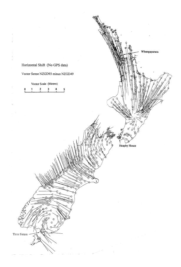
Fig. 1. Current distortions in NZGD 1949 [Taken from Bevin, A.J. and J. Hall. 1995: The review and development of a modern geodetic datum. *New Zealand Survey Quarterly. Issue 1: 14 - 18.*]
