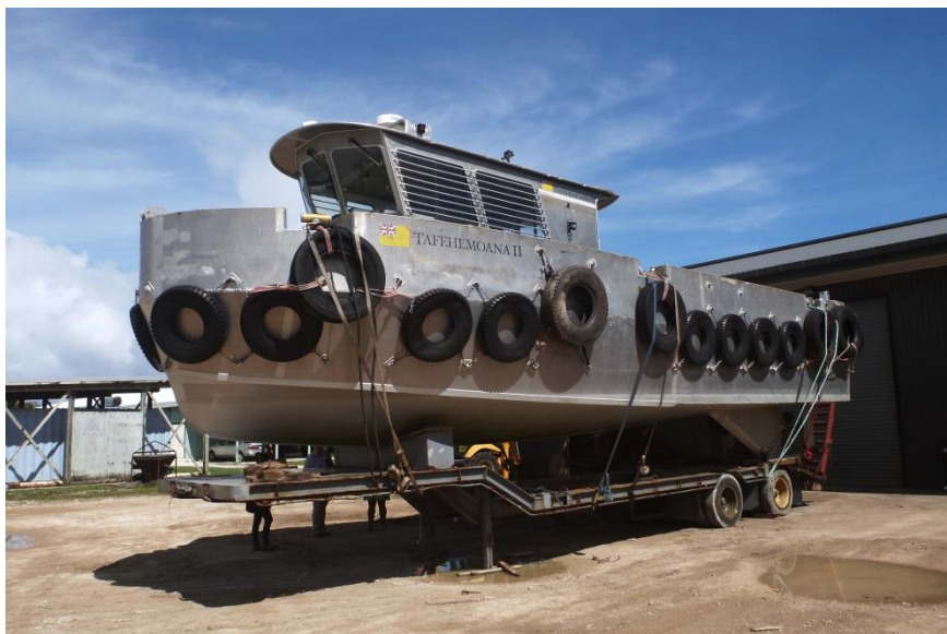
Figure 12: Tafehemoana II used with 13.5 m barge for cargo transfer
