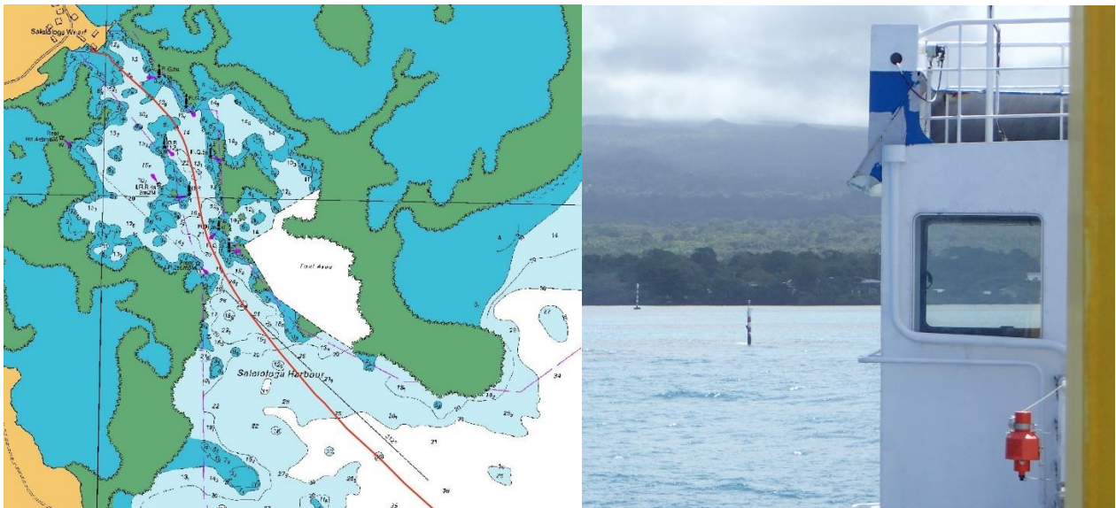
Figure 62: Ship track leaves outer leads open to the south to avoid coral growth close north of the line of leads
