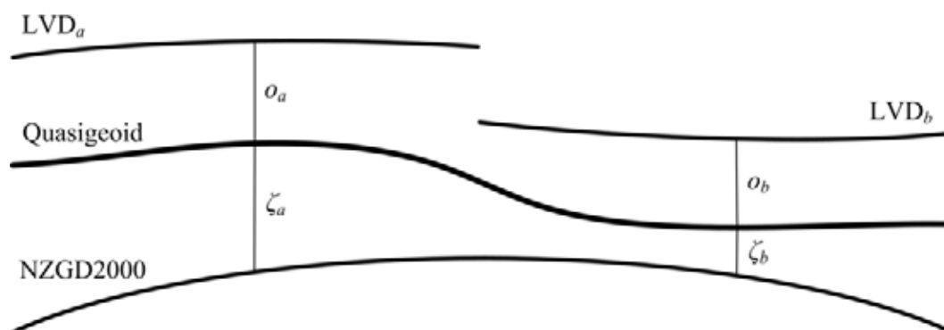
Figure 2.8 Proposed new vertical datum for NZ using a quasigeoid ( \zeta ) and LVD offset ( o ) to relate heights in the 13 normal-orthometric LVDs and the ellipsoidal NZGD2000
