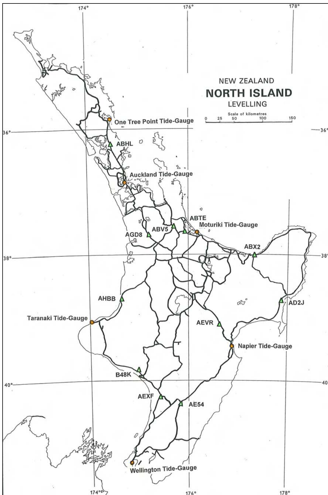
Figure 2.4 NZ North Island precise levelling networks, tide-gauges and vertical datum junction points (adapted from NZNCGG, 1991; Mercator projection)
