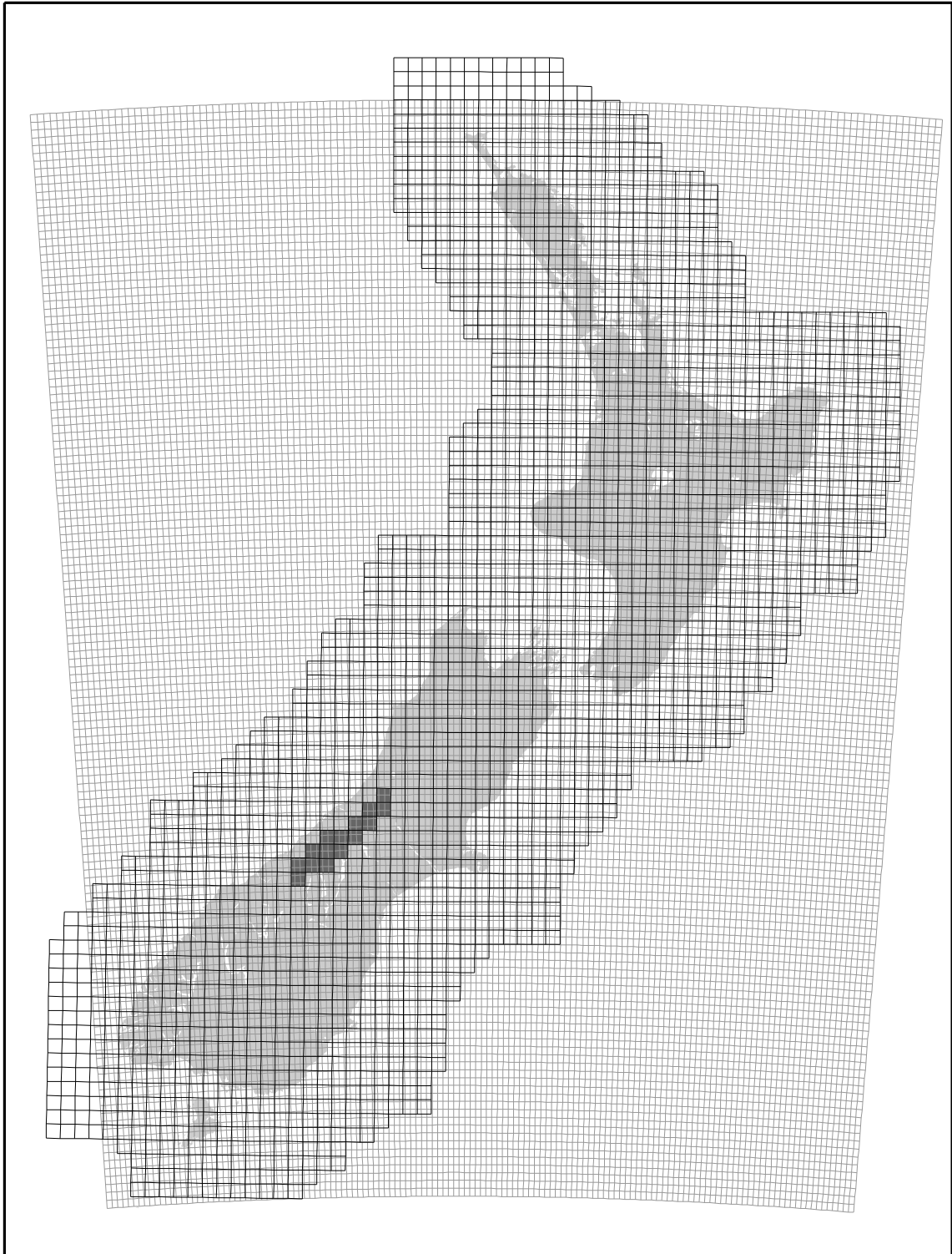
Figure 3: The coarse grid shown is the 20km grid of points on which the distortion model was calculated. The shaded cells are those on which the distortion constraint on the cells was downweighted to account for the difference between the original NZGD49 definition on the east of the South Island and the later extension on the West Coast. The distortion model was interpolated onto the finer grid for publication.
