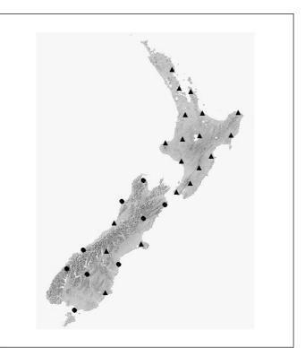
Figure 7. Active control network (Chatham Island excluded). Triangles represent operating stations as at July 2003 and circles planned stations.
