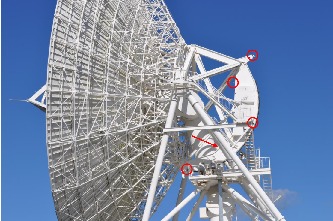
Figure 6.5: Placement of targets on 30 metre dish for the elevation observations. The second target in is obstructed by the telescope frame.
