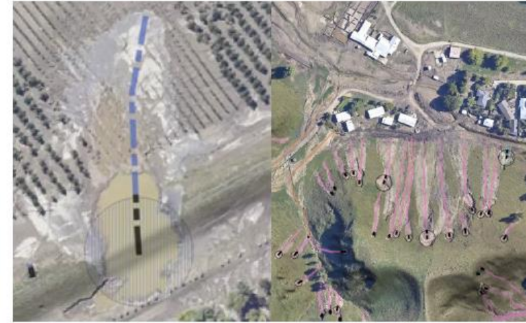
Example of mapped landslides at 1:5000 scale. The first example is a stopbank breach using the 'unclear' movement type
