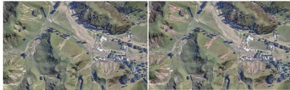
Aerial image showing Ex-Tropical Cyclone Gabrielle landslides (left) with overlaid mapped landslides (right)
