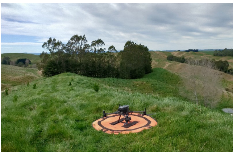
Scion UAV utilising SouthPAN for high-definition forestry mapping.
