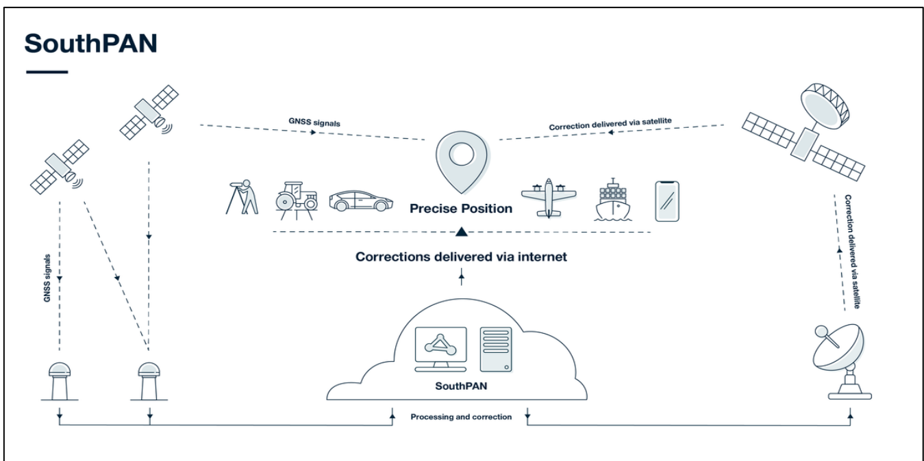
A simplified diagram showing how SouthPAN/SBAS works
