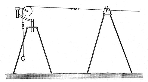
and for moving it horizontally at right angles to the base, so that the tape could be adjusted to touch the mark on the measuring head. The position of the pulley trestles was arranged so that about one-quarter of the length of the cord hung between the pulley and the straining weight and about three-quarters lay between the pulley and the tape. The swivel-hooks prevented any torsion in the cord from causing the tape to twist.
