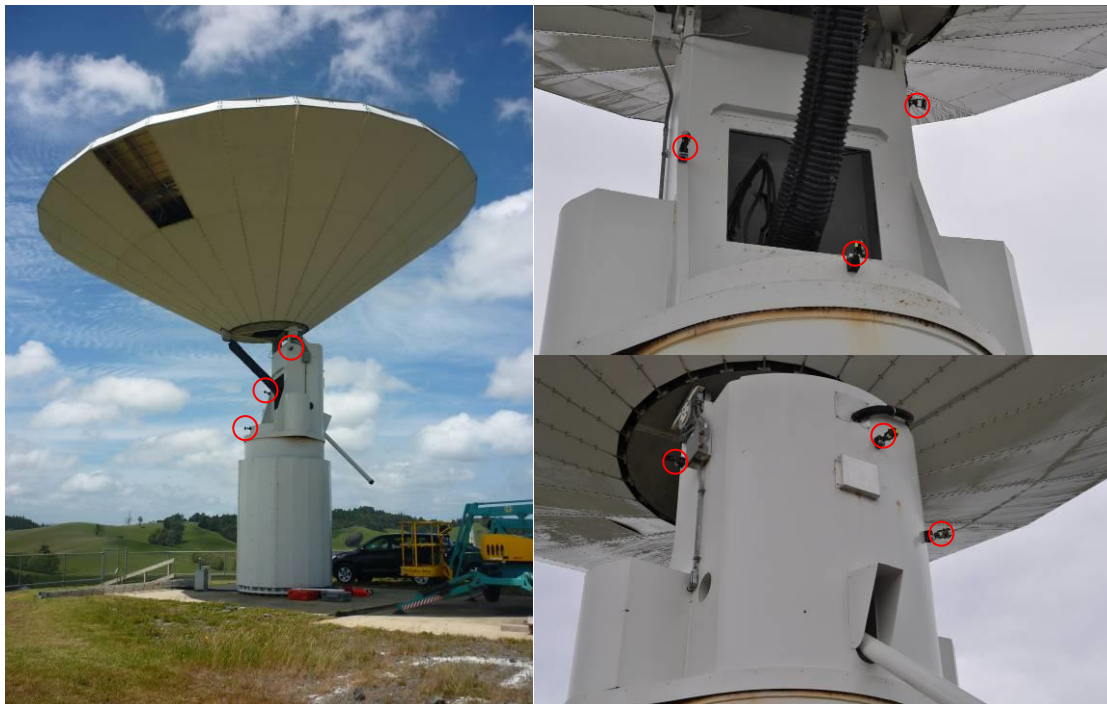
Figure 6.2: Target placement on the front (left and top right) and back (bottom right) on telescope for the azimuth observations.
