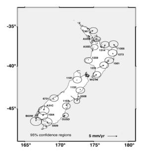
**Fig 4**. Velocity differences and 95% confidence regions for points used in NZGD2000 whose velocities have been updated with 1 to 3 epochs of new data since 1998.
