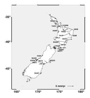
Fig 5. Differences between velocities predicted by the deformation model and velocities observed at continuous sites established since the model was computed, and having > 2 years data. Uncertainties not shown (see Table 2).
