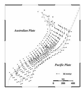
**Fig 1.** NZGD2000 deformation model, with horizontal velocities relative to the Australian plate plotted at the nodes of the model.
