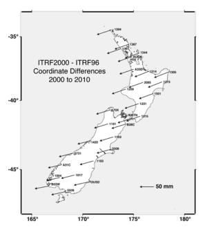
Fig 3. Horizontal coordinate differences between ITRF96 and ITRF2000 from epoch 2000.0 to epoch 2010.0.
