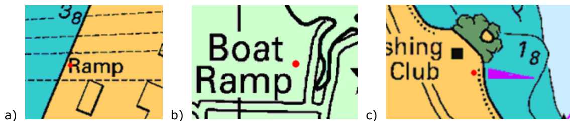
Figure 22: The exact location of the ramp/slipway location is not defined in these representations (a, b and c). The red spot defines where the SLCONS point should be positioned.
