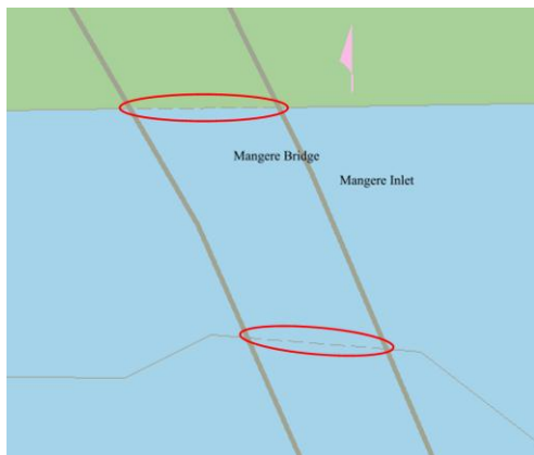
Figure 32: The DEPCNT (dotted line) beneath the bridge has QUAPOS = 4 (approximate) encoded.
