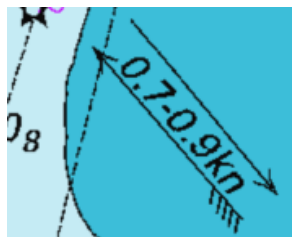
Figure 16: A representation (NZ4633) of flood and ebb tide streams with a range in velocity.
