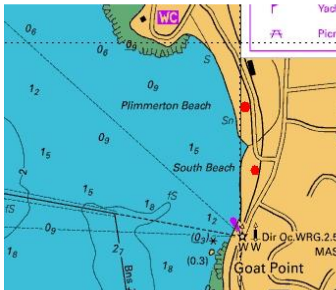
Figure 20: LNDGRN points (red dots) positioned in the most appropriate place on the landward side of the coastline. "South Beach" and "Plimmerton Beach" are captured in OBJNAM.
