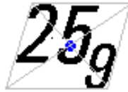
Figure 6: The centre of sounding figures is to be derived as shown here.
