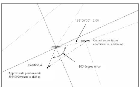
**Figure 4:** Node 39842990 has poor existing Landonline coordinates – its correct position is shown by Position A.
