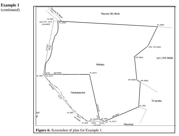
The first test, **Reg 28 and 26.2.c.i: Misclose of obs between boundary marks**, has a failed observation between PEG ML 20689 (id 27480501) and Node ID 27477217 (id 27477217). This observation misclose was reported to be 1.3 times greater than the permitted tolerance. The observation was checked to eliminate any capture or survey error. No such error was found. The failure is therefore assumed to be related to the quality of the source data, which is an 1881 plan.
