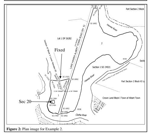
The primary warning message: **Not enough information to calculate node** occurs because the three parcels are not connected. The adjustment selects one node to hold fixed, which in this example is part of Lot 1. As there is no connection between the nodes forming Lot 2 and Section 20, and the fixed node in Lot 1, the adjustment cannot calculate coordinates for nodes in Lot 2 and Section 20. This leads to these nodes being automatically rejected.
