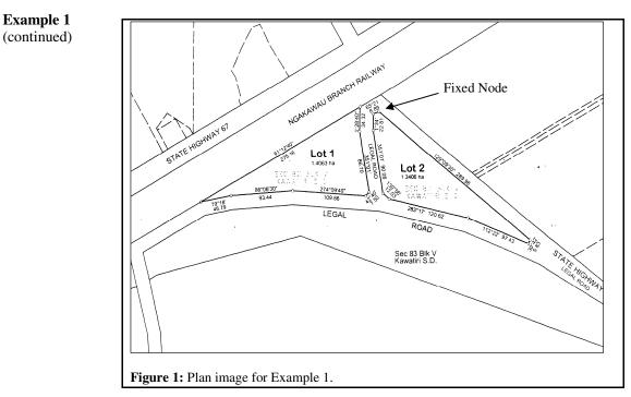
The primary warning message: **Not enough information to calculate node** occurs because the two lots are not connected. The adjustment selects one node to hold fixed, which in this example is part of Lot 2. As there is no connection between the nodes forming Lot 1 and the fixed node in Lot 2, the adjustment cannot calculate coordinates for nodes in Lot 1. This leads to these nodes being automatically rejected.
