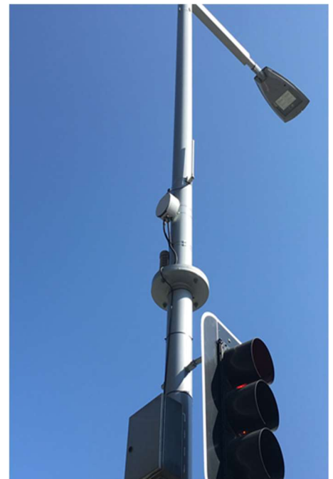
Image 3: Product of the Flexible Sensing Platform – a KITE – installed on a power pole in Christchurch
