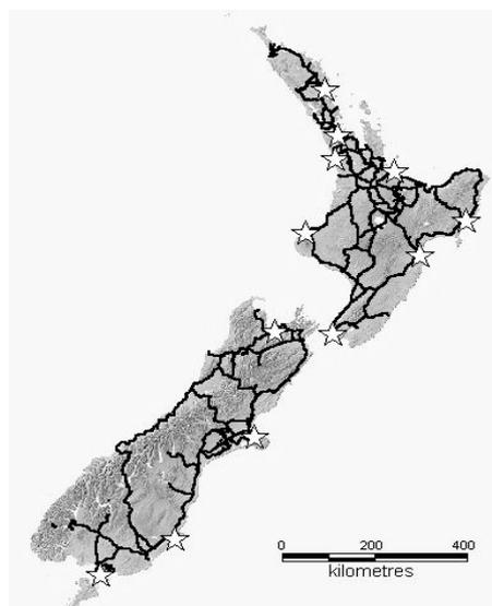
**Figure 1.** Tide gauges and levelling networks used to provide vertical geodetic control in New Zealand
