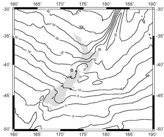
**Figure 3.** The 2002 New Zealand gravimetric co-geoid (contours in metres)
