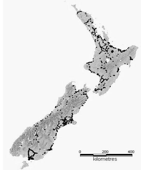
**Figure 4.** The 1017 GPS/levelling data over New Zealand
