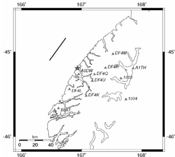
**Figure 5.** Plot of the 11 resurveyed campaign stations in the Fiordland area. The star indicates the location of the earthquake below the surface. The solid black line indicates the location of the ruptured fault projected to the surface.
