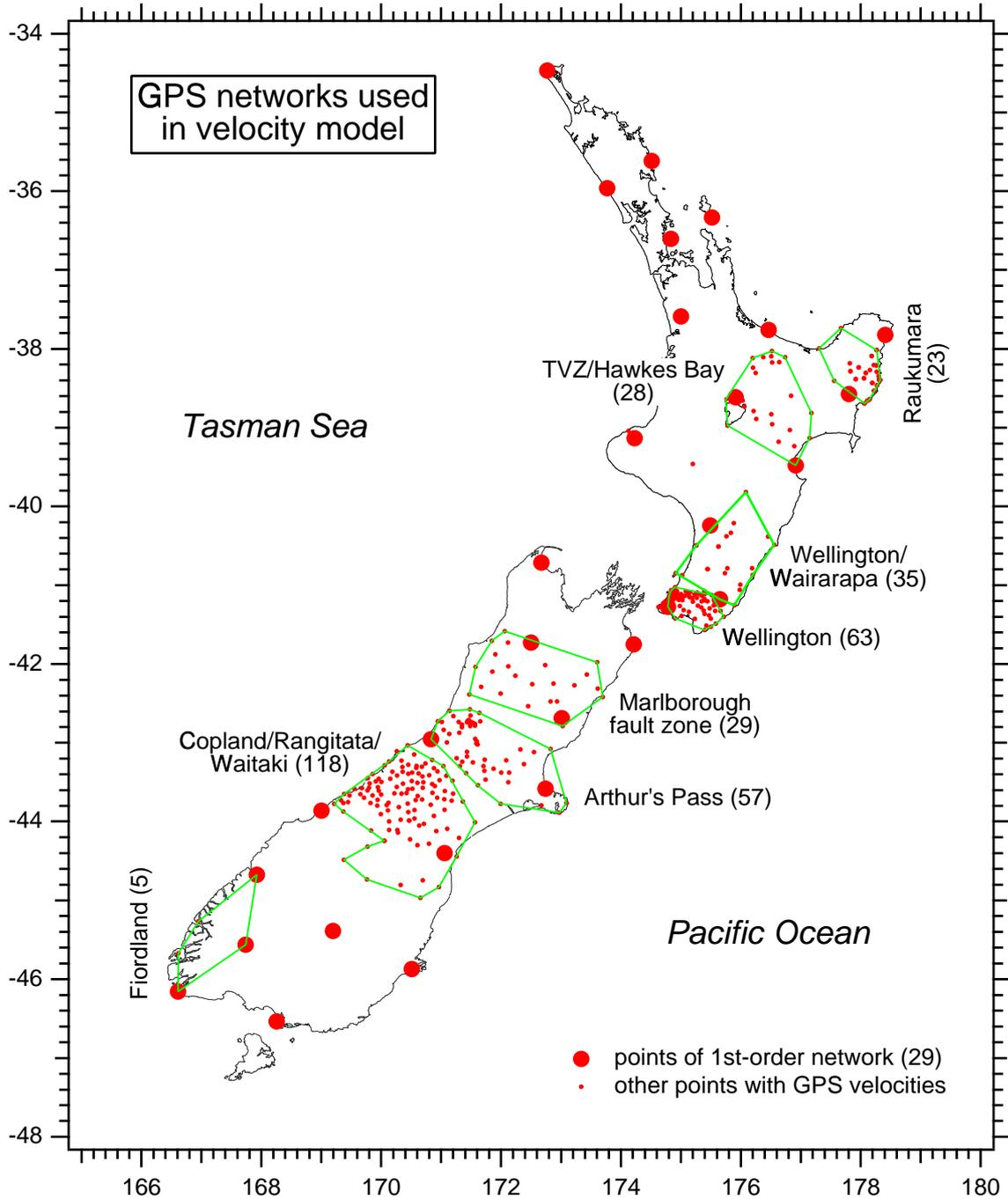
Figure 1 GPS observed marks used to develop the New Zealand Velocity Model
