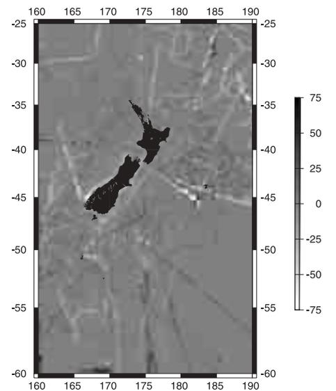
**Figure 1.** Difference between the NCTU01 altimeter grid and the 1,300,266 points in the New Zealand ship-track gravity database (Units in mGal, Mercator projection)
