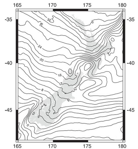
**Figure 5.** The geoid undulations of New Zealand computed from the simple mean free-air gravity anomalies (units in metres relative to EIGEN-EGM. Mercator projection)
