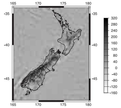
**Figure 4.** The residual reconstructed gravity anomalies over New Zealand (units in mGal relative to EIGEN-EGM, Mercator projection)
