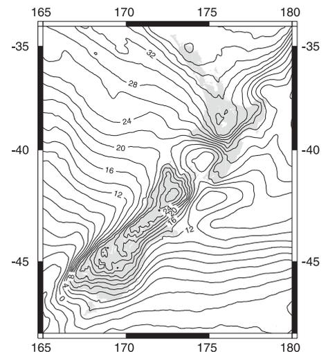
**Figure 6.** The geoid undulations of New Zealand computed from the reconstructed free-air gravity anomalies (units in metres relative to EIGEN-EGM. Mercator projection)
