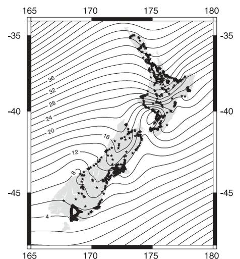
**Figure 2.** The geometrical 'geoid' (in metres) of New Zealand derived using the shown 1055 GPS-levelling heights (Mercator projection)
