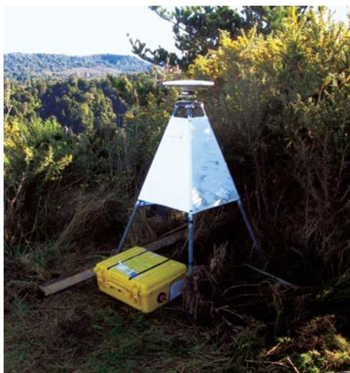
GPS set up for a geodetic survey
