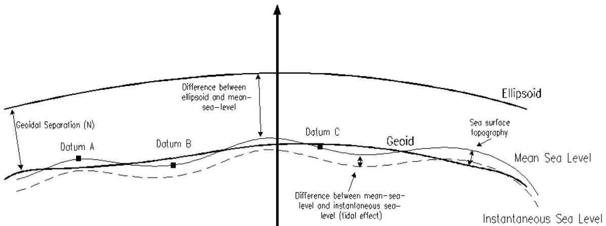
Figure 1. Relationship between ellipsoid, geoid (equipotential surface proposed for new datum), mean sea level (surface on which current datums are based), and instantaneous sea level.
