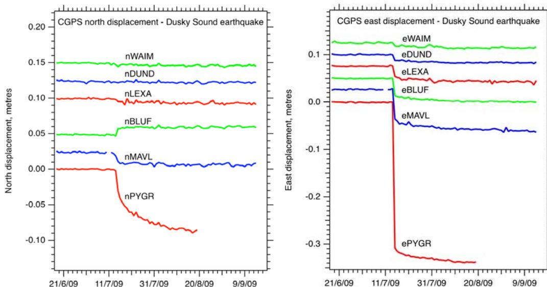
Figure 1: Displacement at CGPS stations (Bevan et al. 2009)
